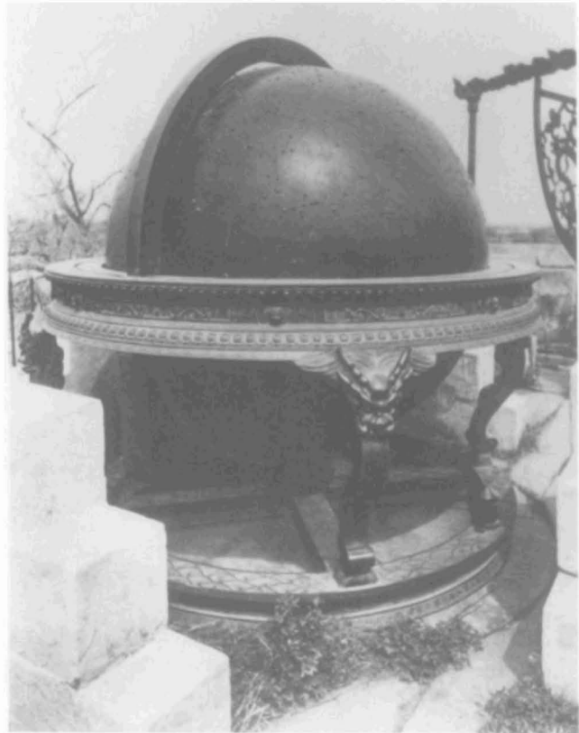
FIG. 13.42. VERBIEST'S CELESTIAL GLOBE IN BEIJING. One of the many instruments cast by Verbiest that can still be seen at the Ancient Observatory, Beijing, this celestial globe is still in almost pristine condition (above and right). Diameter of the original: ca. 1.5 m. Ancient Observatory, Beijing. Photographs from Zhongguo Shehui Kexueyuan Kaogu Yanjiusuo, Zhongguo gudai tianwen wenwu tuji , 104 and 105.
