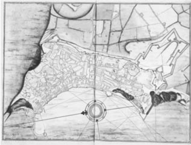
FIG. 27.13. ANCONA, SURVEY PLAN, JACOMO FONTANA, 1585–90. One of a very limited number of orthogonal plans realized in the sixteenth century and the basis for two project presentation drawings. Fontana had made a model of the city in the 1560s when he served as gunner for the papal forces, and the survey on which the model was based may underlie this drawing as well as a perspective plan that he published in 1569. Size of the original: 36.5 × 49.7 cm. Photograph © BAV (Vat. Lat. 13325, fol. 11v–12r).
