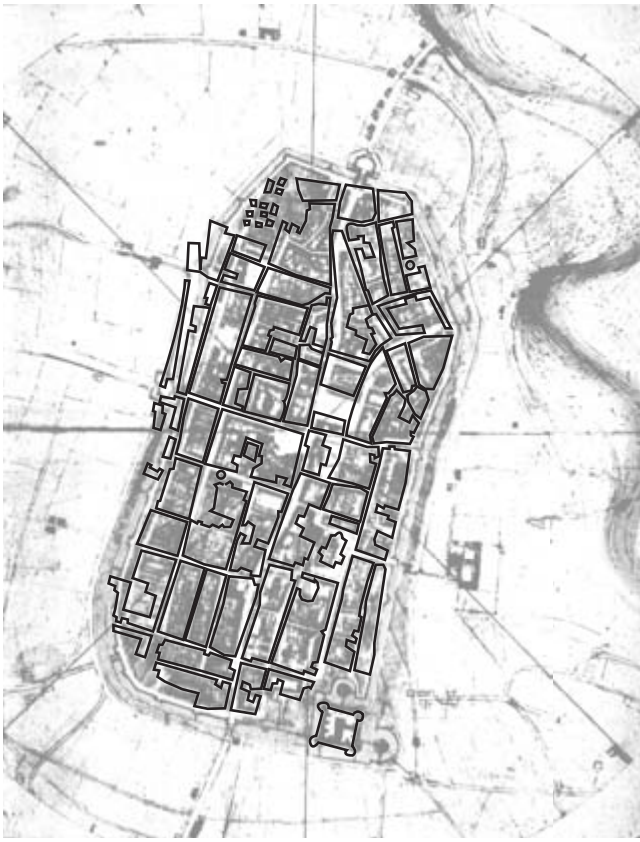
FIG. 27.1. IMOLA, LEONARDO DA VINCI, 1502. A modern survey has been laid over the sixteenth-century plan. The comparison shows that Leonardo did not always capture the shape of the plan, and that often when his survey differs from the plan on the ground, it has the apparent intention of improving the plan's formal composition. Leonardo executed the drawing in connection with a commission from Cesare Borgia to examine the papal fortresses of the Romagna. He inscribed it inside a circle whose perimeter is divided into eight winds, each with eight subdivisions. Inscriptions to the right and left of the circular plan give (inaccurately) bearing and distance to neighboring towns. See figure 36.16.
