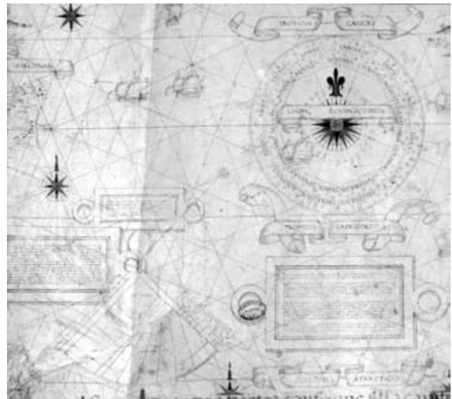
FIG. 40.3. DETAIL FROM THE WORLD MAP OF DIOGO RIBEIRO, 1529. This detail shows a quadrant and circular figure for finding solar declination, both with accompanying instructions. The text in the boxes explains how to read solar declination off of the figure and the accompanying latitude scale (given the date), how to use the quadrant, and how to calculate latitude given the solar declination and the sun's height at noon. Similar illustrations and explanations appear on several of Ribeiro's other world maps. The complete world map is shown in figure 30.29. Size of the original: 80 × 204.5 cm; size of the detail: ca. 57 × 64 cm. Photograph © Biblioteca Apostolica Vaticana, Vatican City (Borgiano III).
