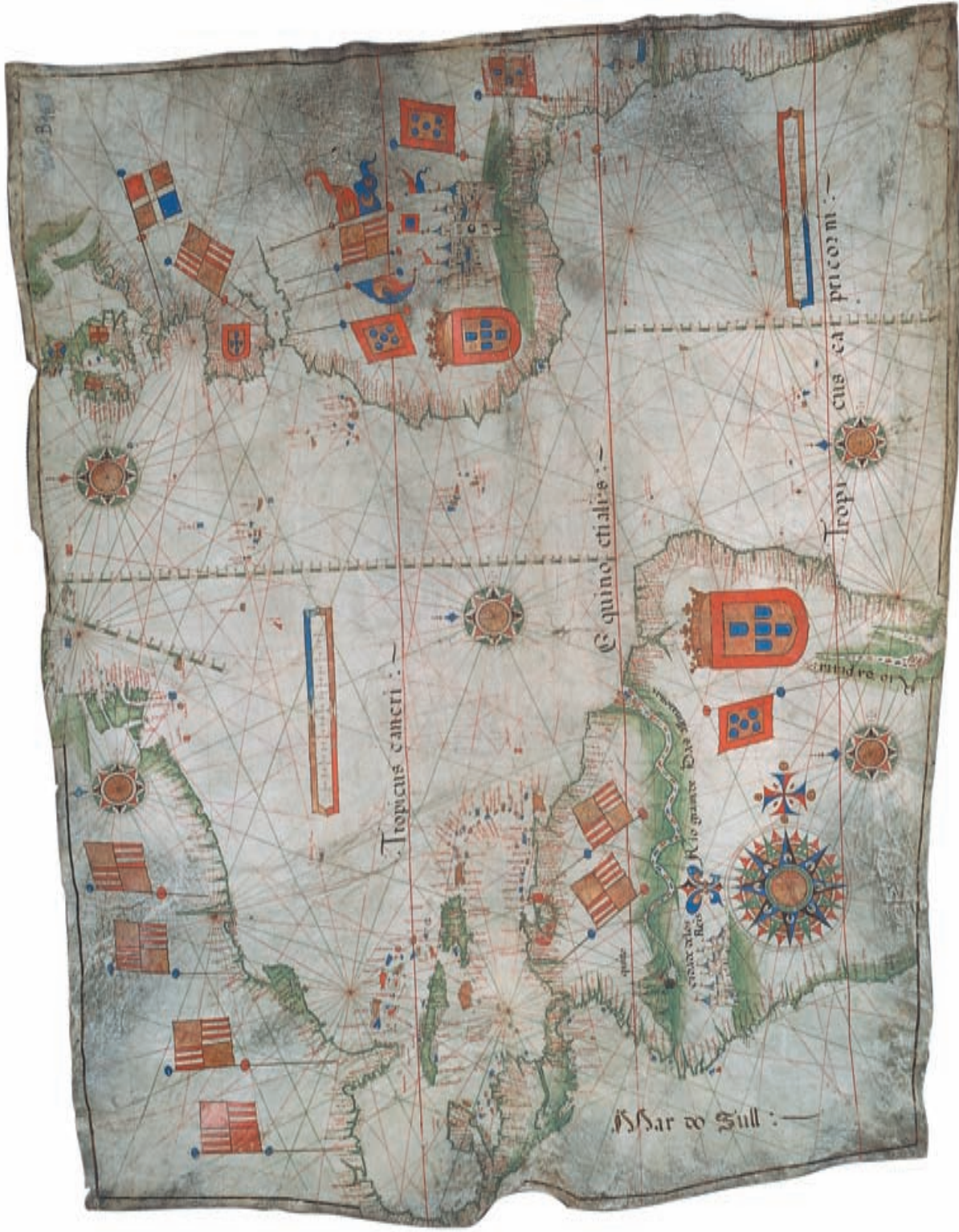
PLATE 14. PLANE CHART OF THE ATLANTIC OCEAN, CREATED AFTER 1549 BY AN ANONYMOUS PORTUGUESE CARTOGRAPHER. (See p. 519.) The chart's latitude scale is prominently depicted in the middle of the ocean. Significantly, this chart also has an oblique meridian, located just off of the Labrador coast. Size of the original: 63 X 88 cm. Photograph courtesy of the BNF (Cartes et Plans, Rés. Ge B 1148).
