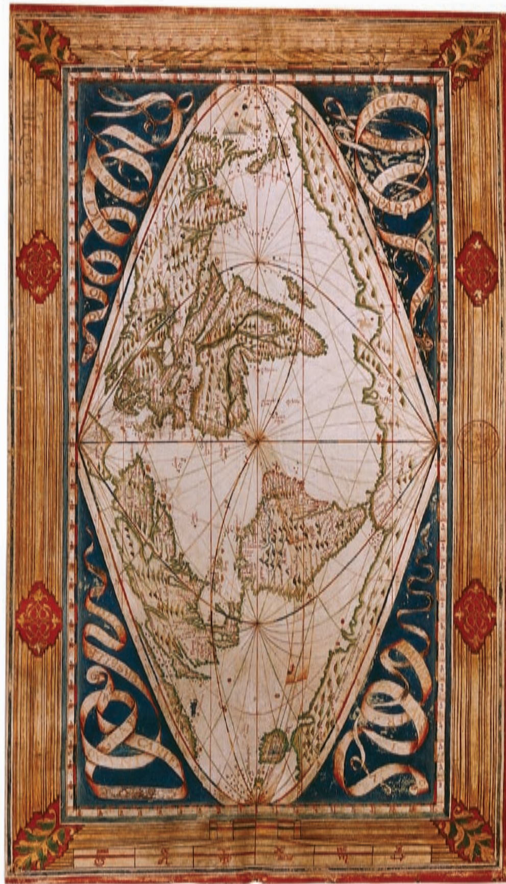
PLATE 12. JEAN COSSIN, MANUSCRIPT WORLD MAP ON THE SINUSOIDAL PROJECTION, 1570. (See p. 372.) This projection, based on elegant sine curves, is an equal-area
