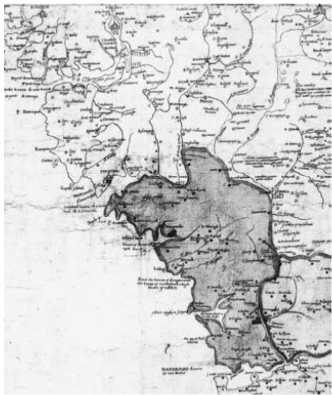
FIG. 55.4. ROBERT LYTHE, DETAIL FROM MAP OF CENTRAL AND SOUTHERN IRELAND, 1571. The whole map shows the exact area that Lythe is known to have surveyed himself and appears to be in his own hand. The tinted broken lines are county boundaries. This region was not surveyed again until the middle of the seventeenth century. Size of the entire original: 81 × 112 cm. Photograph courtesy of Lord Egremont and the West Sussex Record Office, Chichester (PHA 9581).
