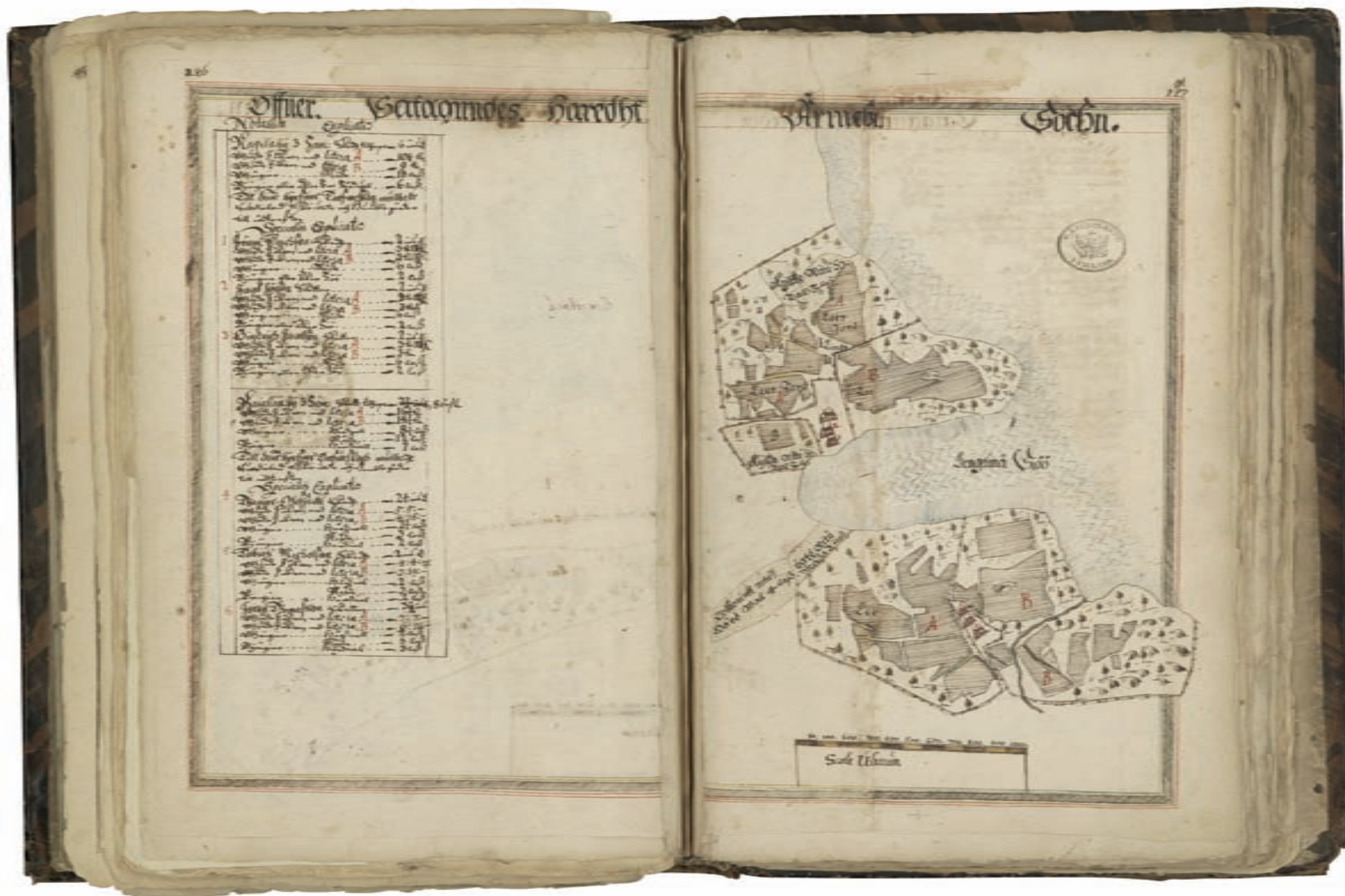
PLATE 74. ANDERS STRENG, NAAPPILA AND RAJALAHTI, ORIVESI PARISH, FINLAND, 1634. (See p. 1804.) A sample of the first generation of geometrical maps ( geometriska kartor ) produced by the Landmäterikontoret. The scale is in Swedish alnar (1:15,000), and color is also used. The Nota-
