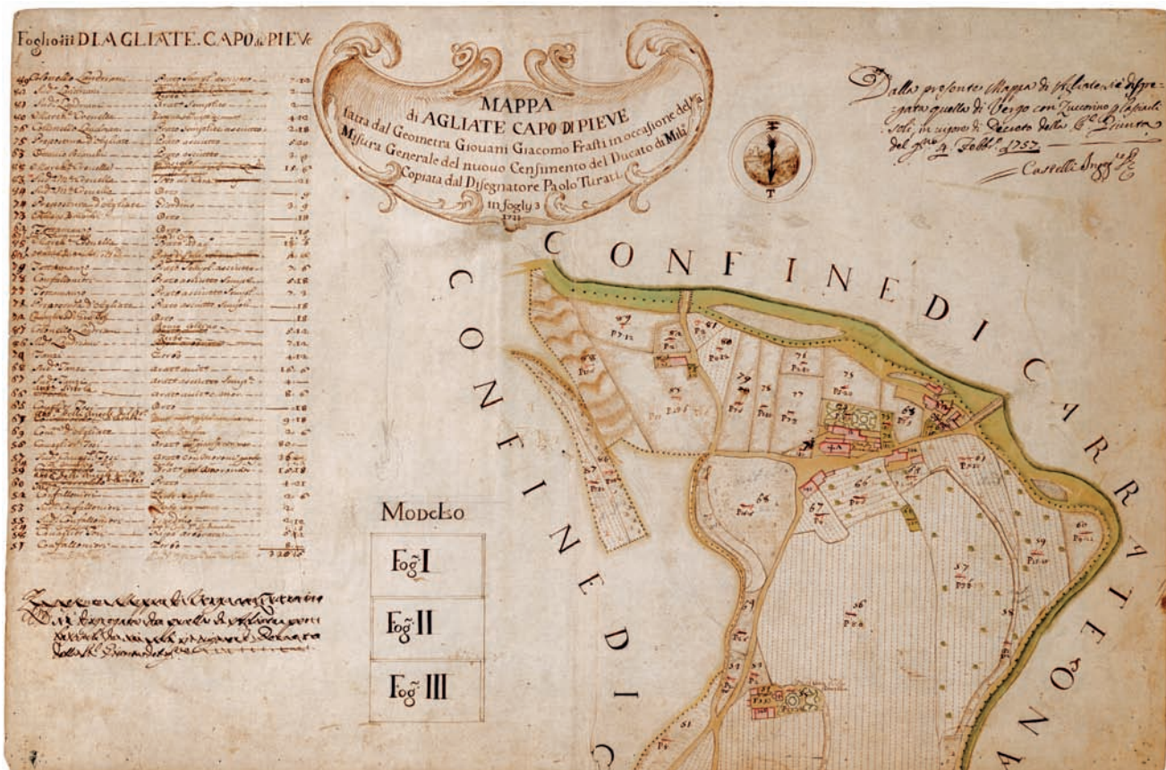
FIG. 648. PORTION OF GIOVANI GIACOMO FRASTI, “MAPPA DI AGLIATE CAPO DI PIEVE,” 1722, 1:8,000. Upper sheet of three from one of the manuscript fair copies of each comune reduced from field work at 1:2,000 in the Milanese censimento , 1720–23, made for levying land tax.
