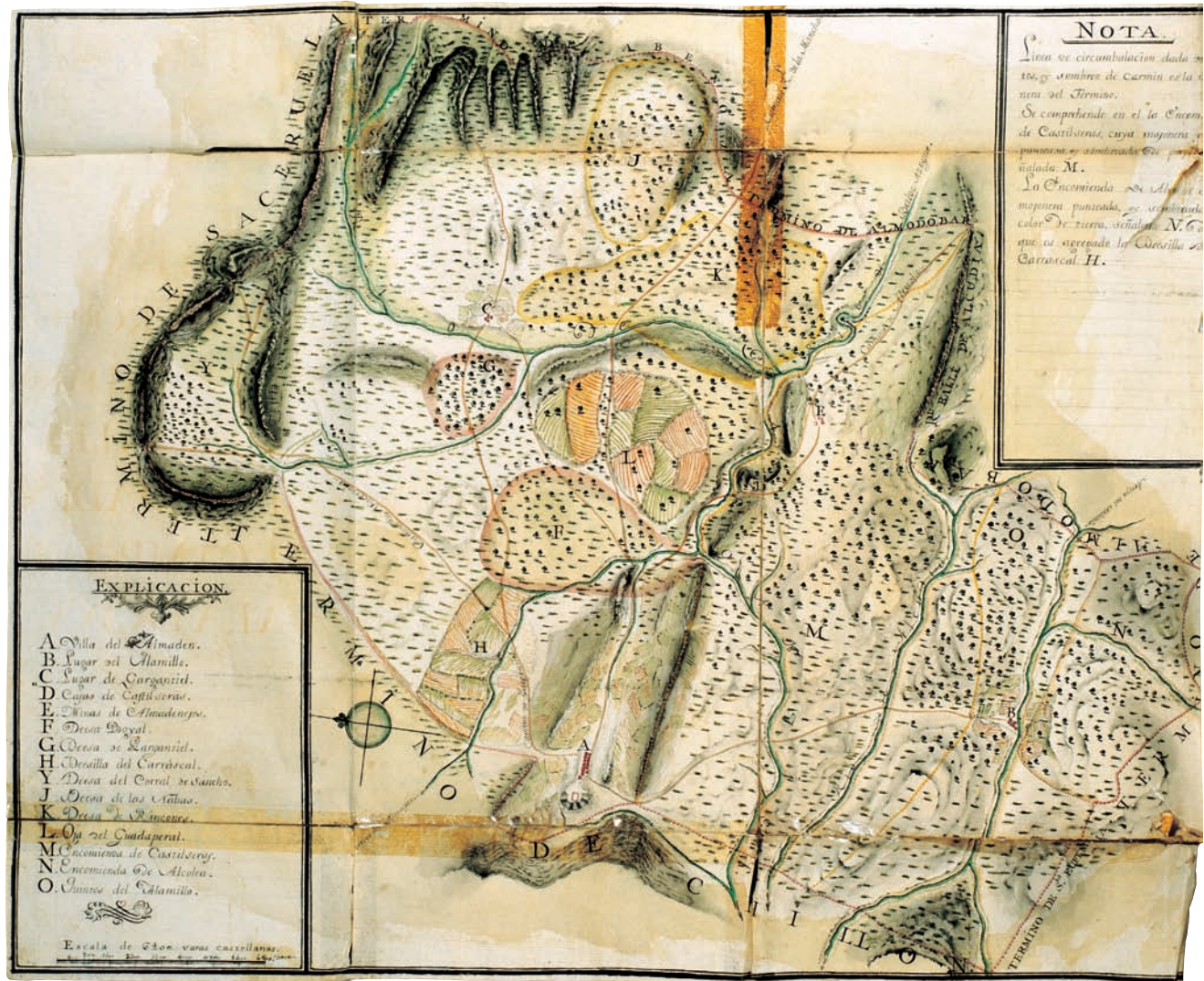
FIG. 690. MAP OF ALMADÉN, 1751, FROM THE CATAS- TRO DE ENSENADA. This manuscript is the only geomet- rically surveyed map in the Catastro de Ensenada. It has a graphic scale in the lower left corner representing 6,400 varas castellanas (1 vara castellana = ca. 0.83 m), a color key (noted in the box top right), and an explanatory key for the letters on the plan. This map was probably created because it was the
