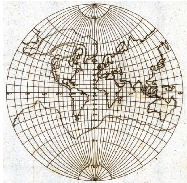
FIG. 645. LAMBERT'S CONFORMAL PROJECTION OF THE EARTH WITHIN A CIRCLE, NOW KNOWN AS THE LAGRANGE PROJECTION. From Lambert 1772, pl. 6, fig. 11.
