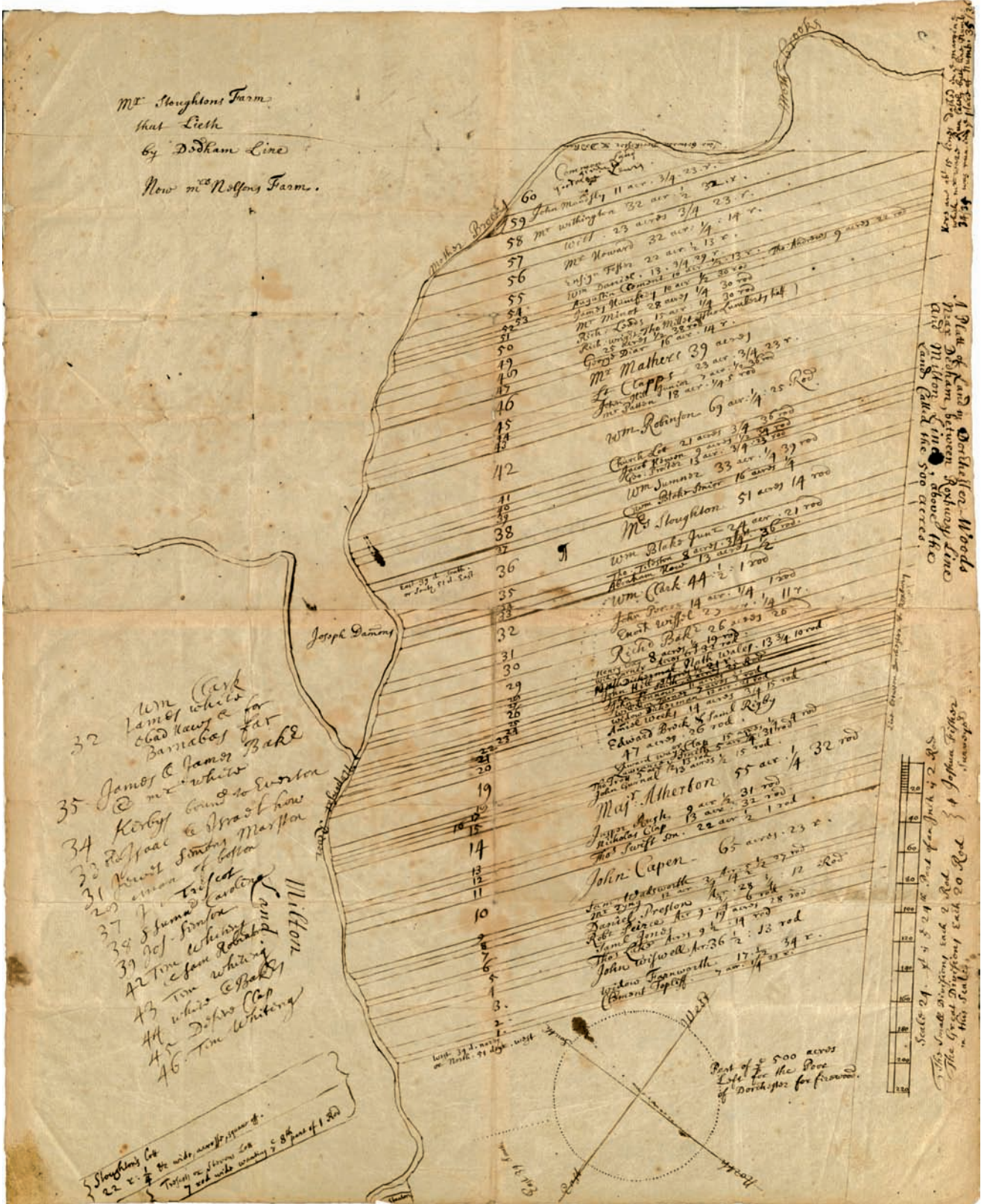
FIG. 674. JOSHUA FISHER, "A PLATT OF LAND IN DORCHESTER WOODS NEAR DEDHAM," CA. 1670. Manuscript, ink on paper, 1:9,500. This plat illustrates the subdivision of five hundred acres of common land in Dorchester, Massachusetts, into sixty long lots for proprietary share-
