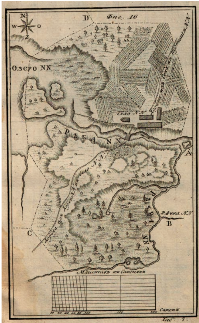
FIG. 686. DMITRIY PAVLOVICH TSITSIANOV, KRATKOYE MATEMATICHESKOYE IZ"YASNENIYE ZEMLEMERIYA MEZHEVOGO (ST. PETERSBURG, 1757), PL. 7. The illustration in this seminal printed survey manual shows local surveyors how to render different types of landscape. © The British Library Board, London.
