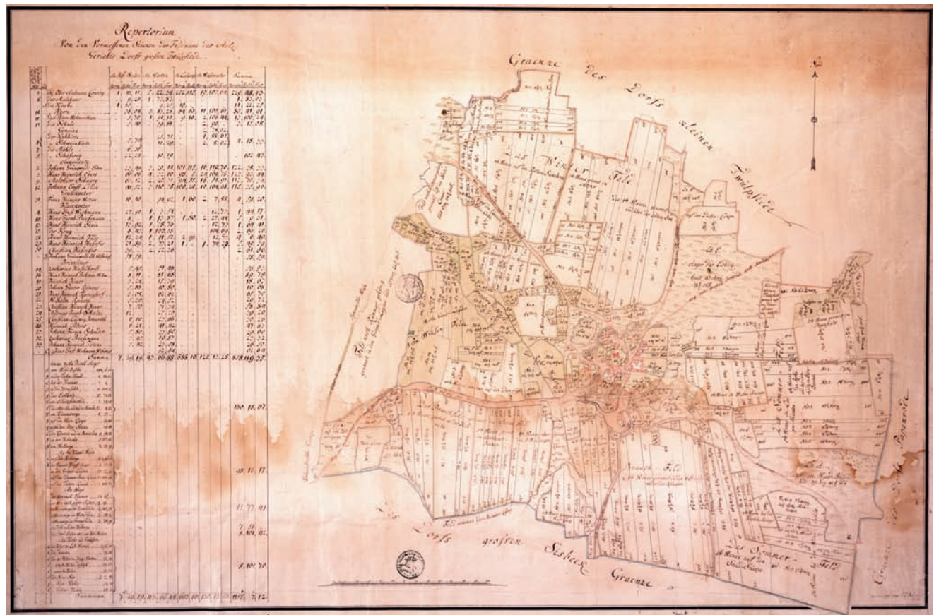
FIG. 647. MAP OF GROß TWÜLPSTEDT DRAWN IN 1758. Part of the Braunschweigische Landesvermessung enclosure and agrarian reform survey. The scale is 1:4,000. The manuscript map shows the cadastral situation after consolidation.
