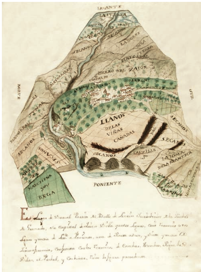
FIG. 689. MAP OF DÚRCAL, 1752, FROM THE CATASTRO DE ENSENADA. This manuscript map typifies the cadastral plan drawn “as it appears to view” with no scale and no key. The cardinal points are identified and the nature of the landscape incorporated in the colors, shading, and tree symbols. Size of the original: 31 × 20 cm. España, Archivo Histórico Provincial de Granada (Catastro de Ensenada. Dúrcal. Libro 1.213).
