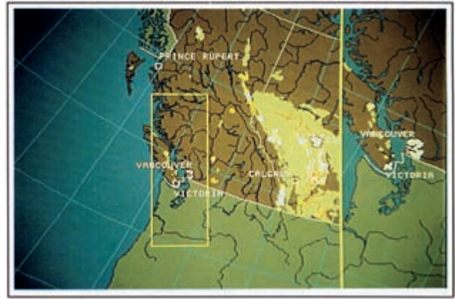
FIG. 61. RULE-BASED AUTOMATIC GENERALIZATION IN THE CANADIAN ELECTRONIC ATLAS MARK 1 , AN EARLY ELECTRONIC ATLAS PROTOTYPE SYSTEM. The system was able to automatically convert area symbols into point symbols when, during the scale reduction process, an area became too small for acceptable legibility standards. This detail is from a Lexidata 3400 computer display. Image courtesy of Eva Siekierska.
