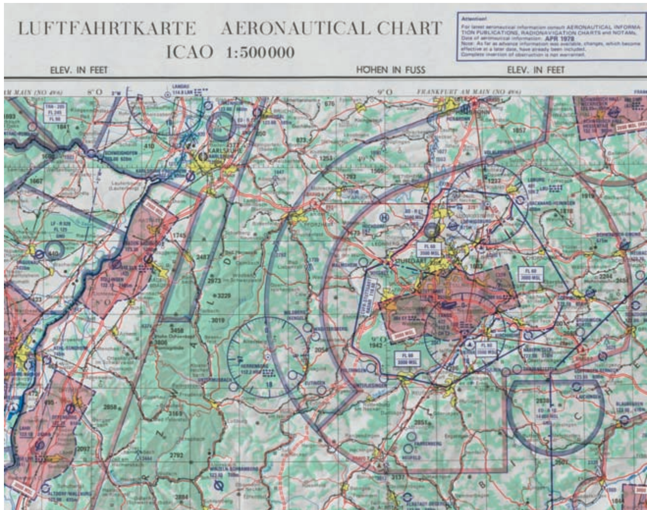
FIG. 15. DETAIL FROM THE INSTITUT FÜR ANGEWANDTE GEODÄSIE, LUFTFAHRTKARTE AERONAUTICAL CHART ICAO 1:500,000, STUTTGART (NO 47/6) , 15TH ED., MARCH 1978. Published in Frankfurt am Main by the Bundesanstalt für Flugsicherung. Title and detail of Germany's standard visual navigation chart with radio navigation facilities, air traffic controls (tinted blue and red), and airspace restrictions; produced according to standards issued by the International Civil Aviation Organization (ICAO).
