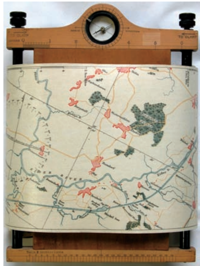
FIG. 10. UNTITLED AIR NAVIGATION STRIP MAP OF THE KAISER WILHELM CANAL (KIEL CANAL), ROYAL NAVY AIR DEPARTMENT, 1 JUNE 1915. Published in London by the Hydrographic Department of the Admiralty, 1:506,880. Mounted on British War Department aviator roller chart holder with compass (London: Houghton-Butcher, 1915). One of the first strip maps designed specifically for air navigation, with compass rose. Size of the entire original: 14 \times 142 cm. Image courtesy of the Ralph E. Ehrenberg Collection.
