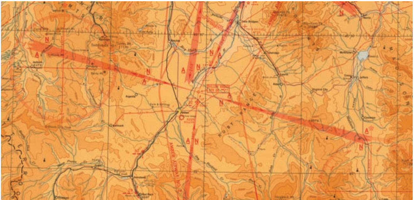
FIG. 12. DETAIL FROM YELLOWSTONE PARK (W-3) , DECEMBER 1940. Published in Washington, D.C. by the USC&GS, 1:500,000. The first modern aeronautical chart series combined visual and radio navigation with the introduction of the Civil Aeronautics Authority's innovative radio range stations that transmitted in Morse code the letters A
