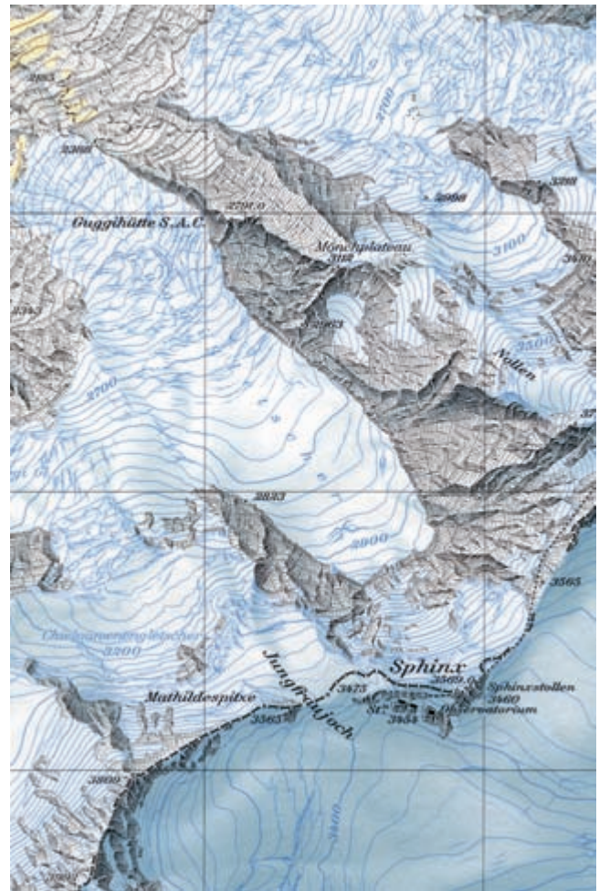
FIG. 30. DETAIL FROM THE LANDESKARTE DER SCHWEIZ 1:25000, FINSTERAARHORN , 1974. Published by the Eidgenössische Landestopographie, Wabern-Bern (sheet no. 1249), this detail of an official Swiss map includes the Jungfrauoch, a well-known peak in the Bernese Alps of Switzerland, and illustrates the artistic emphasis on rock drawing while minimizing contour lines. Size of the original: 53.8 × 73.7 cm; size of detail: 12.7 × 8.4 cm. © swisstopo. Reproduced by permission of swisstopo (BA13119).
