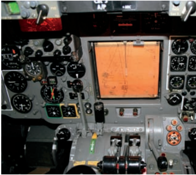
FIG. 18. PICTORIAL DISPLAY CHART MOUNTED ON INSTRUMENT PANEL OF A RESTORED HAWKER SIDDELEY HS-121 TRIDENT 3B AIRCRAFT, MANCHESTER AIRPORT. An example of an interchangeable spool loaded moving map operating in conjunction with Decca Navigator, a hyperbolic radio navigation system of ground transmitting chains, by a pioneer of pictorial presentation of navigation data. Image courtesy of Neil Lomax.
