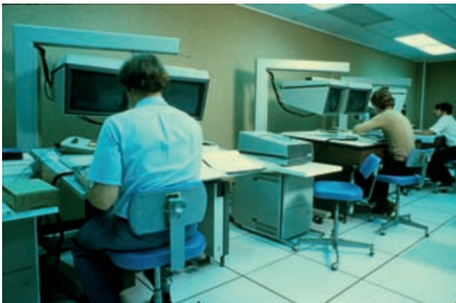
FIG. 224. M&S DIGITIZING AND EDITING EQUIPMENT, CA. 1978. M&S Computing Inc. (now Intergraph Corporation) DDES (digital data editing system) was used for manual digitizing of printed maps and for interactive correction of digitizing errors. Image courtesy of the U.S. Geological Survey.
