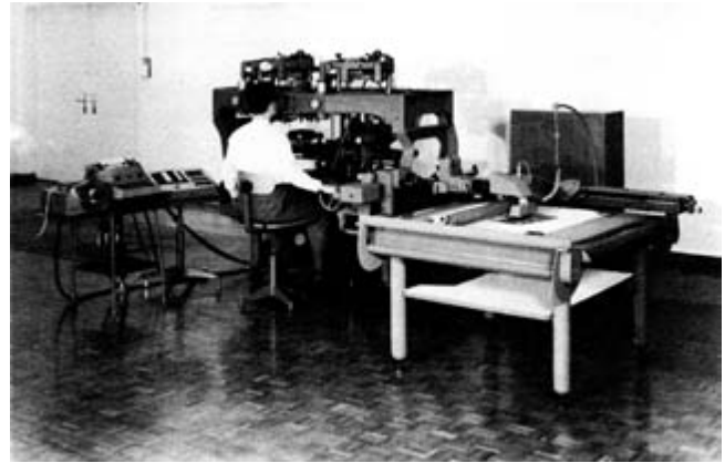
FIG. 231. THE WILD HEERBRUGG LTD. AUTOGRAPH A7 STEREOPLOTTER. Optical stereoplotters were used to extract geographic data and plot maps from aerial photograph stereo pairs. Proficient operation of the device required extensive training and experience. As indicated by the photograph, the plotter was a large machine relative to the size of the stereo pairs that it processed (ca. 9" × 9", or 23 cm × 23 cm). From Blachut and Burkhardt 1989, 121 (fig. 73). Copyright by the American Society for Photogrammetry and Remote Sensing.
