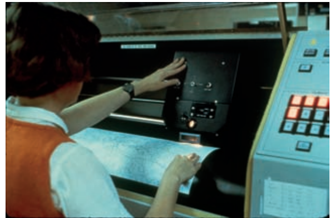
FIG. 225. MAP BEING LOADED ON A SCITEX DRUM SCANNER, CA. 1984. This scanner was used to digitize feature separates from USGS 1:100,000 scale topographic maps as part of the production program that led to the creation of TIGER. Image courtesy of the U.S. Geological Survey.
