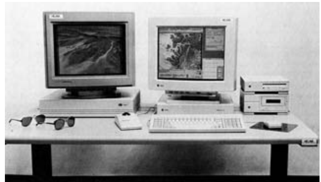
FIG. 232. DIGITAL PHOTOGRAMMETRIC WORKSTATION. These stations made optical and analytical photogrammetric devices effectively obsolete by the end of the century. The combination of high accuracy, small size, relatively low cost, and ease of use gave the new systems a competitive advantage. From Lillesand and Kiefer 1994, 350 (fig. 4.30). Permission courtesy of John Wiley & Sons, Inc.
