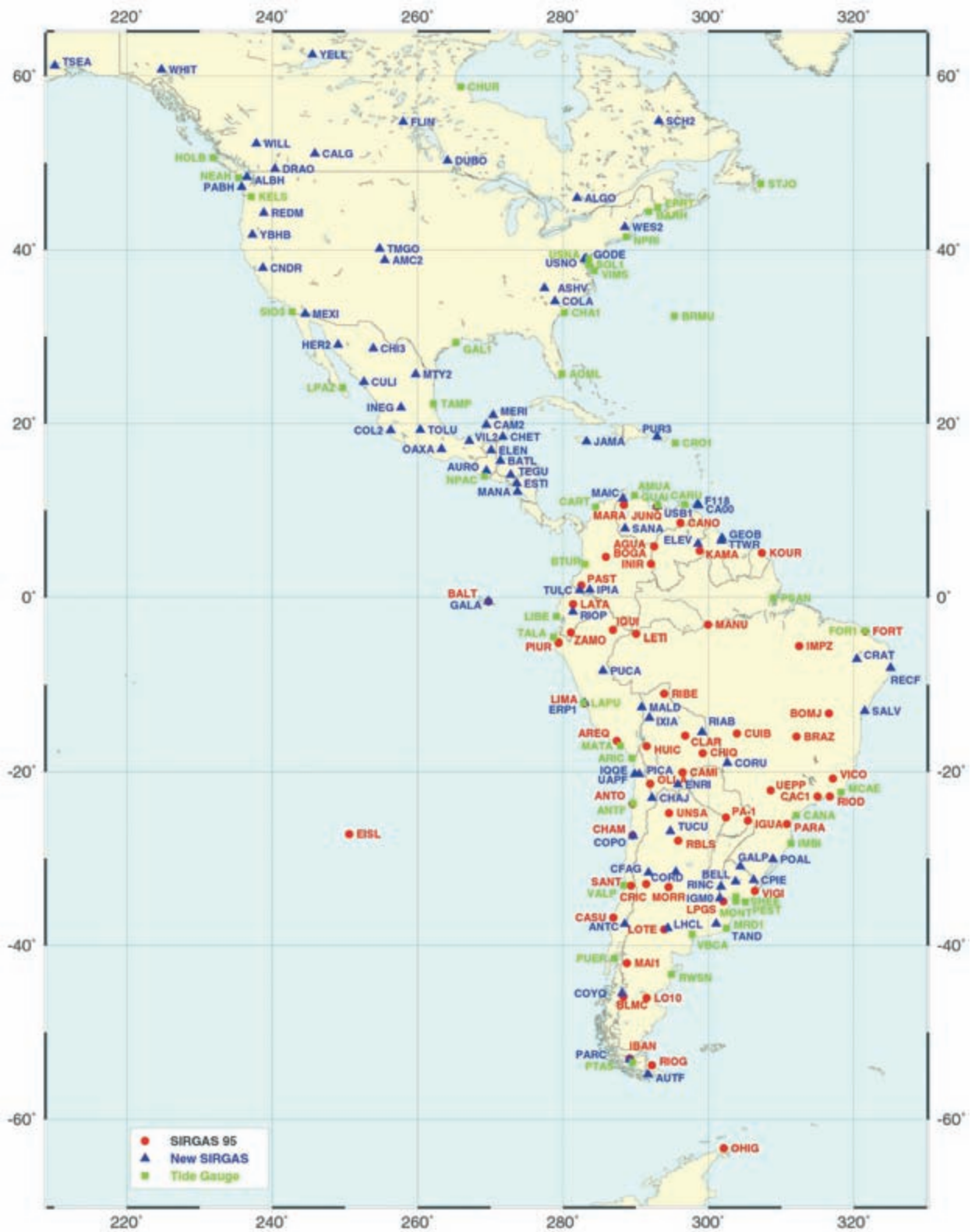
FIG. 294. THE GEOCENTRIC REFERENCE SYSTEM FOR THE AMERICAS, SIRGAS 2000 GPS CAMPAIGN STATIONS (TOTAL 184).
