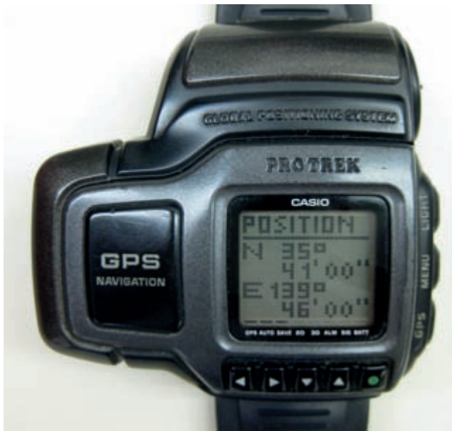
FIG. 337. FIRST GPS WRISTWATCH, PRO TREK. Sold by Casio in 1999 for $895; ten years later GPS watches were no larger than their non-GPS counterparts and cost just over $100. Size of the watch body: 6.5 \times 6.5 cm.
