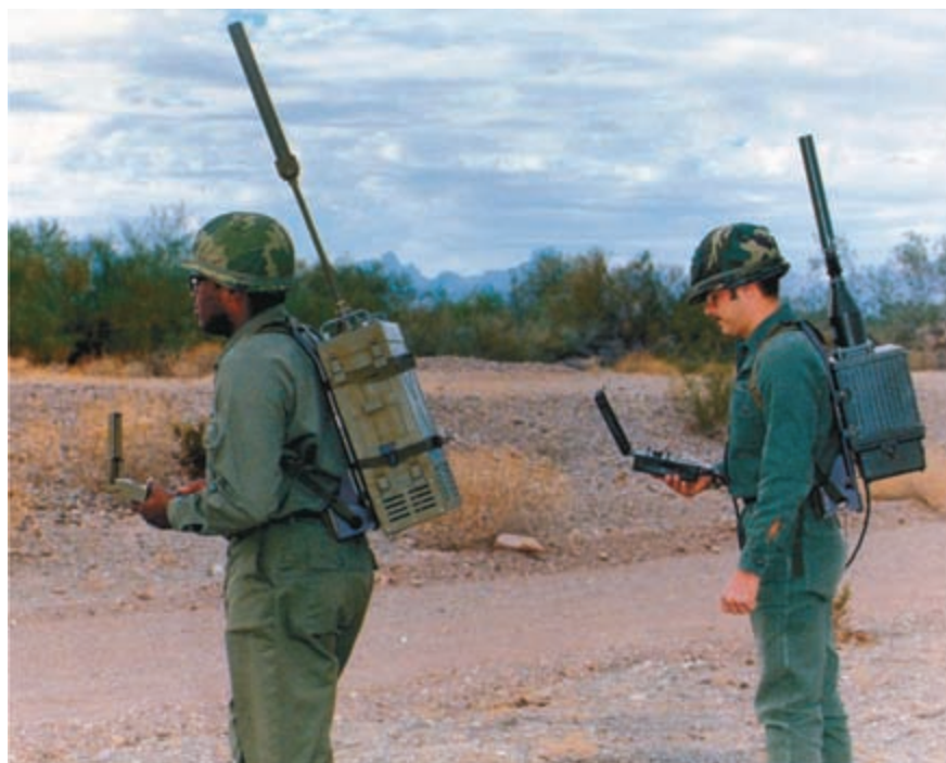
FIG. 336. GPS RECEIVERS IN THE FIELD, CA. 1978. In 1973 the designers of GPS had hoped to eventually produce a portable military receiver weighing less than twelve pounds (5.5 kg). The Manpack of 1978 (left) weighed 14 kilograms, while the Defense Advanced GPS Receiver (DAGR) of 2004 (right) weighed about 400 grams and fit comfortably in the hand.
