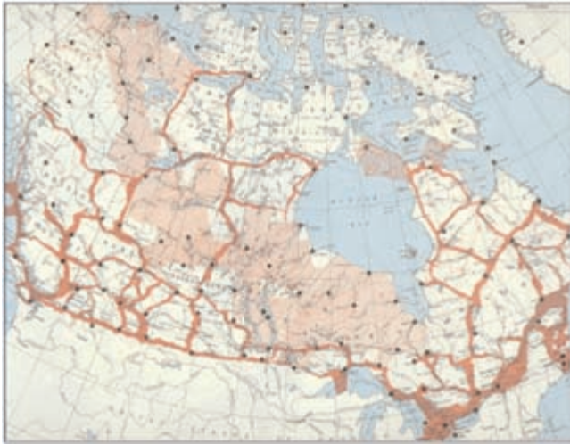
FIG. 292. CANADIAN TRADITIONAL HORIZONTAL CONTROL NETWORK. Central part of the Canada landmass showing much of the 8,000 station primary geodetic framework, comprising triangulation arcs, Aerodist trilateration, and satellite Doppler positions included in the NAD83 continental adjustment.
