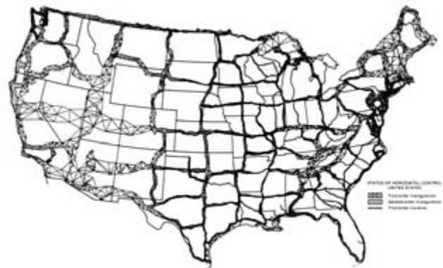
FIG. 291. THE U.S. HORIZONTAL GEODETIC CONTROL NETWORK IN 1927. The categories (top to bottom) are first-order triangulation, second-order triangulation, and first-order trilateration.
