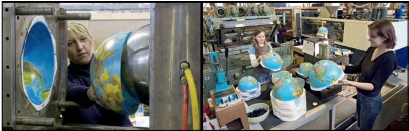
FIG. 345. GLOBE PRODUCTION AT COLUMBUS-VERLAG. Globe hemispheres are produced by a combination of thermoforming and injection molding. Hemisphere being removed from the machine (left) and stacked (right).
