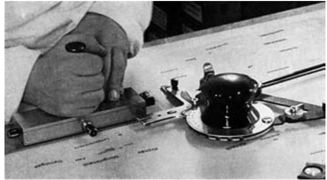
FIG. 449. STAMPING LETTERING WITH THE WULKOW-SCHRIFTSTEMPELGERÄT. Type lettering set in a special holder is being stamped onto a German map using the Wulkow brand of type-stamping equipment. From Bosse 1954–55, vol. 1, between 96 and 97 (fig. 9). Permission courtesy of Elisabeth Seeger Verlag, Freiburg.
