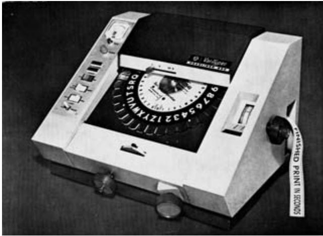
FIG. 452. A LINE OF FINISHED TYPE EMERGES FROM THE VARTYPER HEADLINER 820, A PHOTOCOMPOSER WITH CHANGEABLE TYPMASTER DISKS. The type is produced after being photographed, developed, fixed, and washed within the machine. From A. G. Hodgkiss, Maps for Books and Theses (New York: Pica Press, 1970), 84. Permission courtesy of Robert Hodgkiss.
