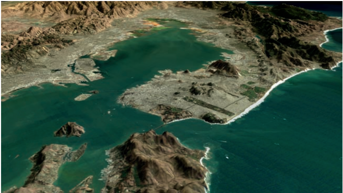
FIG. 462. LANDSAT 5 IMAGE OF SAN FRANCISCO BAY–OAKLAND. Created by combining three bands (1 + 2 + 3 = true color) to make a color image in combination with a digital elevation model with a vertical exaggeration factor of three
