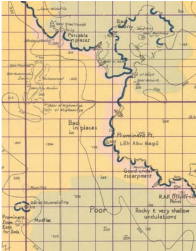
FIG. 542. DETAIL OF A GOINGS MAP OF EGYPT. Khâlda East , 1:100,000, 1942 (sheet 8E). Used to show the nature of the surface and its suitability for traffic, this type of mapping was pioneered in North Africa during World War II. Size of the entire original: 74.0 × 57.4 cm; size of detail: 14.4 × 11.4 cm. Image courtesy of Peter Collier.
