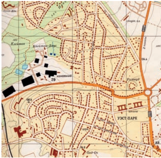
FIG. 577. DETAIL FROM THE 1:10,000 PLAN OF LEEDS, ENGLAND (SHEET 1). Compiled in 1971 and issued in 1972. Note that the widths of roads vary abruptly; some major roads are shown at less than true width, while minor roads are enlarged. The z-bend shown in the east-west (orange) main road at a road junction has never existed and is a compilation error. One of the minor roads shown just south of that is fictitious and other errors are identifiable.
