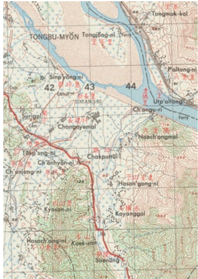
FIG. 601. DETAIL OF AN AMS 1:50,000 MAP, TUKSŎM . Compiled from 1:25,000 sheets, which were based on photogrammetric surveys, this eighth-edition sheet from 1953 (L751, sheet 6626 IV) has place-names in both the Latin alphabet (black) and Korean characters (red). Size of the entire original: 52.9 × 51.0 cm; size of detail: 13.6 × 9.5 cm. Image courtesy of Peter Collier.
