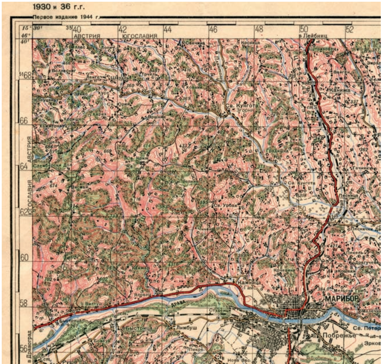
FIG. 574. DETAIL FROM THE FIRST EDITION OF THE 1:100,000 MAP (SHEET L-33-56, MARIBOR). Printed December 1944, it was compiled from the Yugoslav 1:100,000 map of 1932-33 and the Austrian 1:75,000 map of 1937. The
