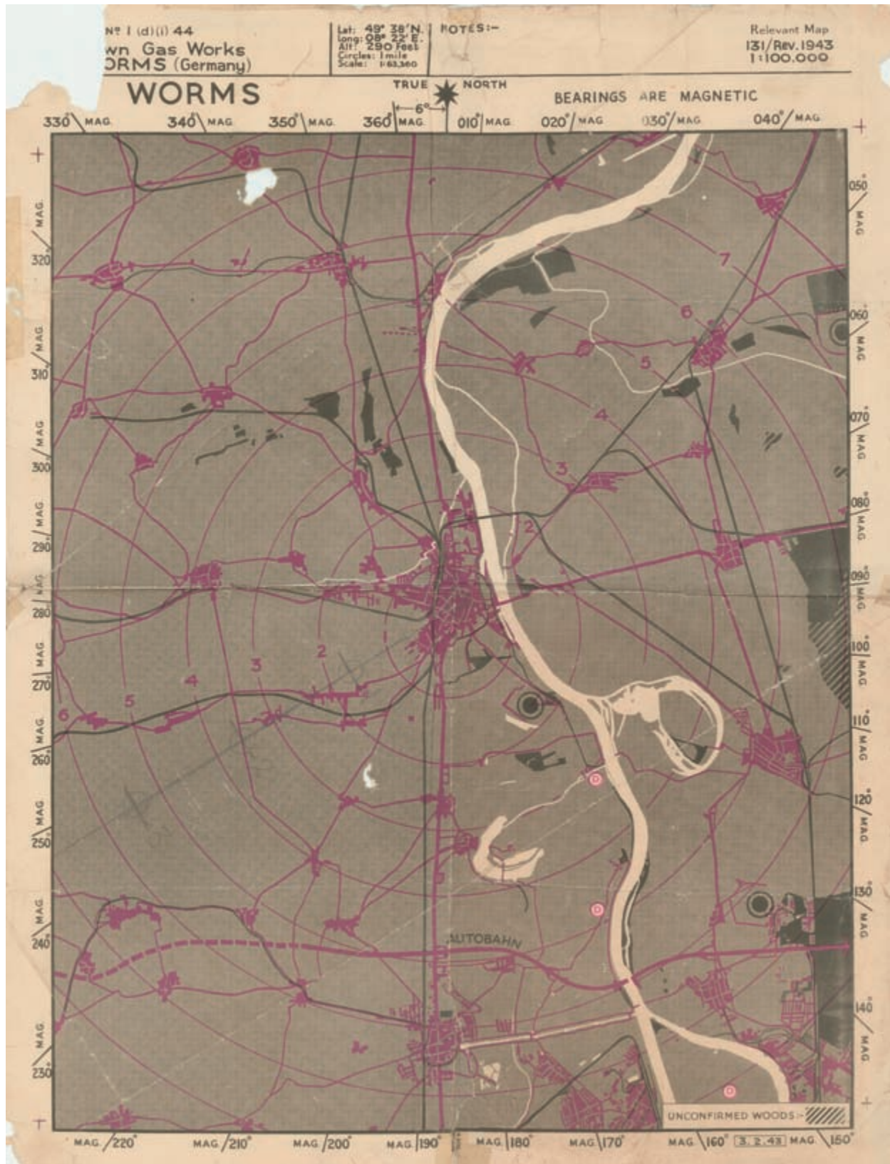
FIG. 544. TARGET MAP OF WORMS, GERMANY, 1:100,000, 1943. Produced for a night bombing raid on Worms gasworks, the coloring was designed to assist navigation and target identification using the H2S radar bomb sight.
