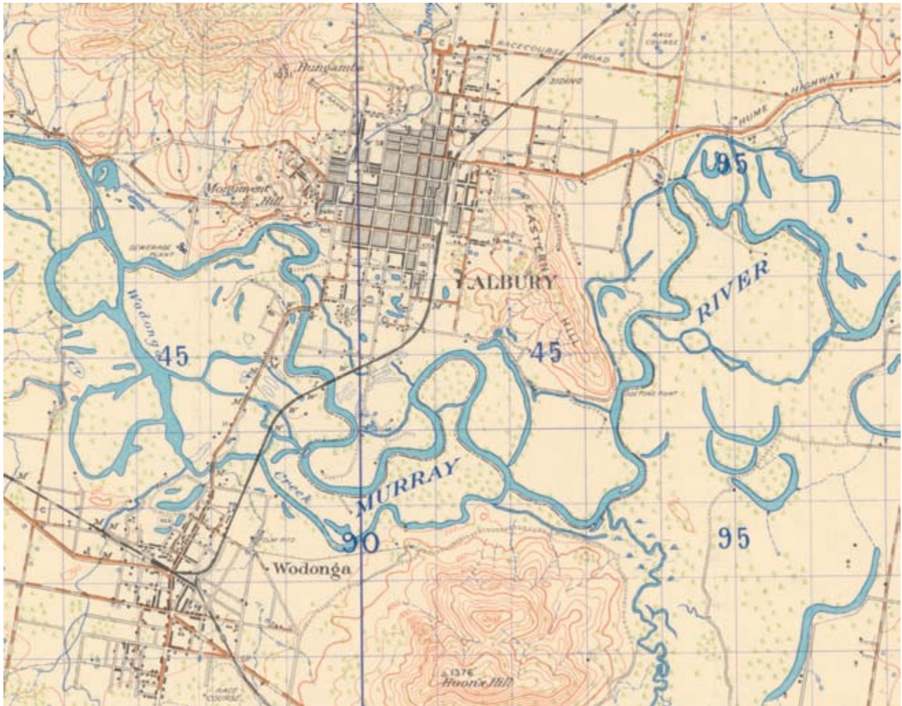
FIG. 602. DETAIL FROM NEW SOUTH WALES AND VICTORIA: ALBURY , JUNE 1933. This is the first map by the Australian military to rely heavily on aerial photography. Surveyed by the Australian Survey Corps and Royal Australian Air Force, prepared by the Australian Section Imperial General Staff, scale 1:63,360.
