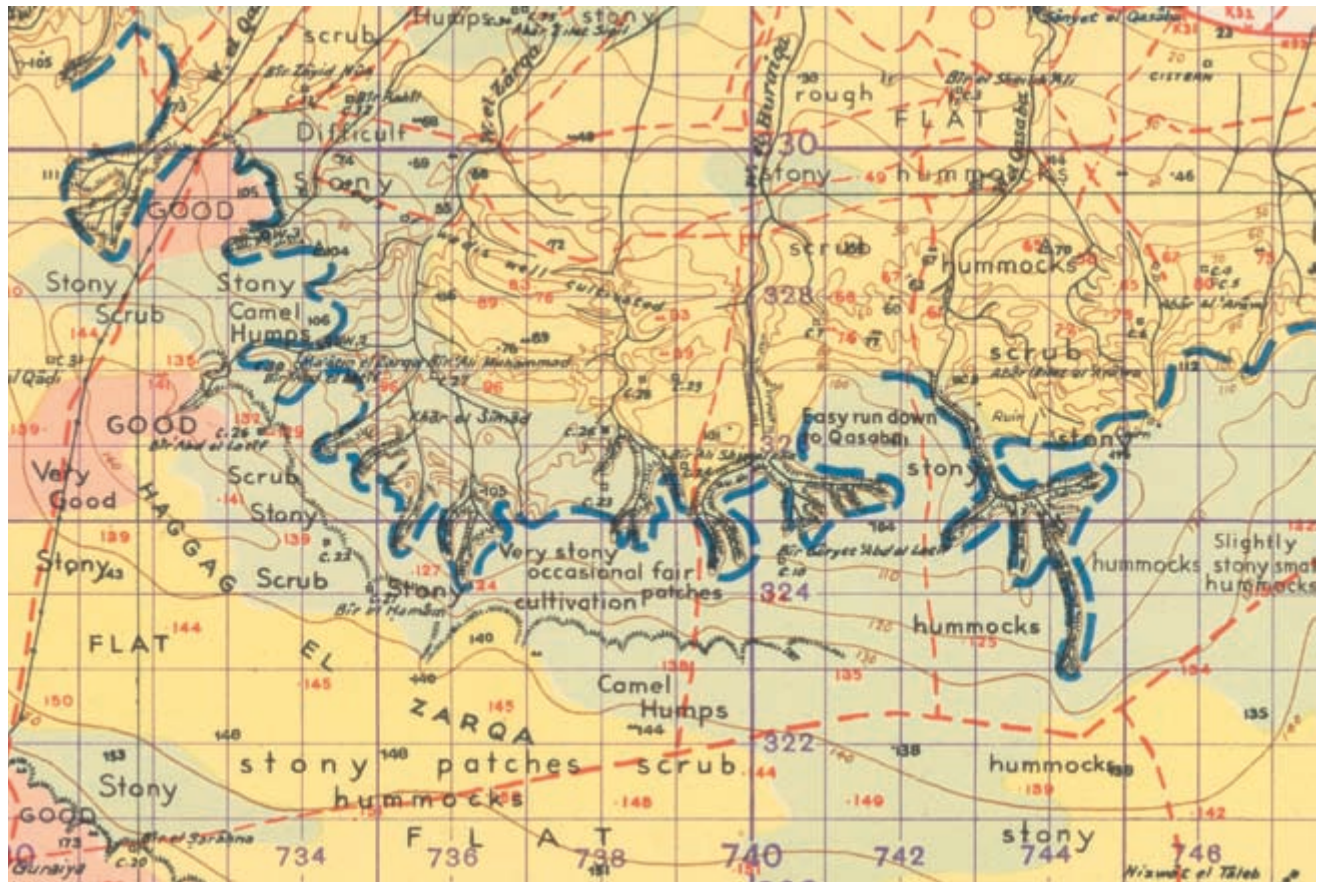
FIG. 583. DETAIL FROM 1:100,000 GOINGS MAP OF MA-TRUH EAST (EGYPT), 1942 (SHEET 3E). The Goings maps were intended to show the suitability of terrain for the movement of mixed mechanized forces.
