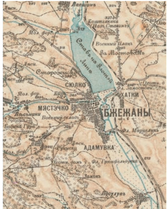
FIG. 590. DETAIL FROM BZHEZHANY, 1917, A RUSSIAN REPRODUCTION OF AN AUSTRIAN 1:75,000 MAP WITH CYRILLIC ADDED. Copying captured enemy maps was very common in wartime. If the map had been acquired prior to the war, it would probably have been redrawn at a Russian map scale.
