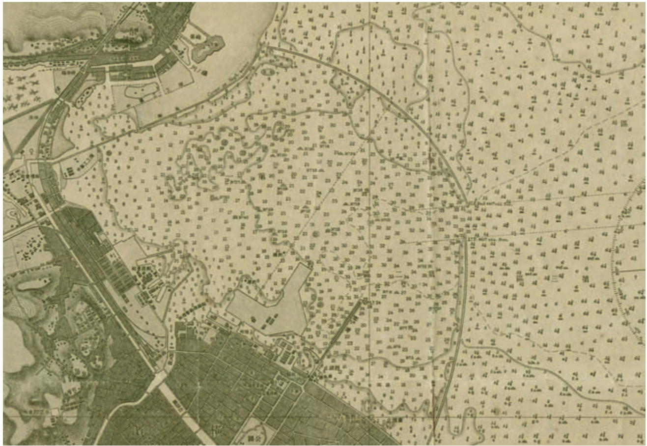
FIG. 515. DETAIL FROM CHART NO. 66, YOKOHAMA AND APPROACHES, 1898. Major corrections, October 1909, scale 1:18,201. JHD soundings in fathoms outside the breakwater. Soundings inside the breakwater are in feet and were engraved by the Ourdan engraving machine.
