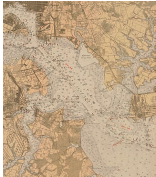
FIG. 506. DETAIL FROM 1931 EDITION OF APPROACHES TO BALTIMORE HARBOR , 1:40,000. U.S. Coast and Geodetic Survey, chart 549. Land is now shown in a buff tint, and larger-scale chart coverage is mentioned as a parenthetical “(chart 545)” in red. Red buoy hulls are also colored. Curves are made to stand out through “sanding,” i.e., use of a stipple pattern. Also of note is the area just above the center labeled “AIRPORT being filled .”
