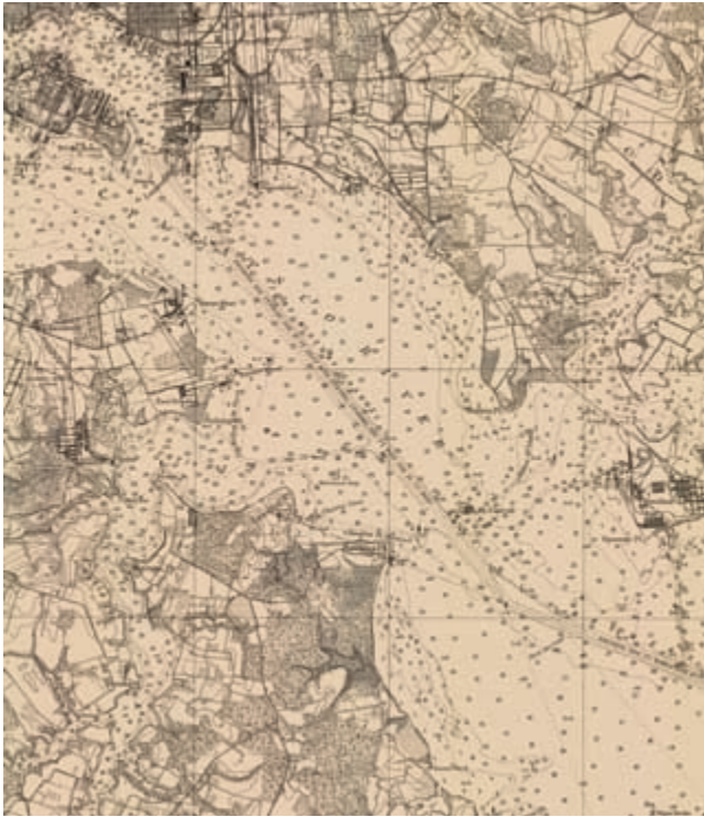
FIG. 505. DETAIL FROM 1900 EDITION OF APPROACHES TO BALTIMORE HARBOR , 1:40,000. U.S. Coast and Geodetic Survey, chart 549. Note the number of projection graticule lines in use and the amount of detail shown on land as well as the lack of color.
