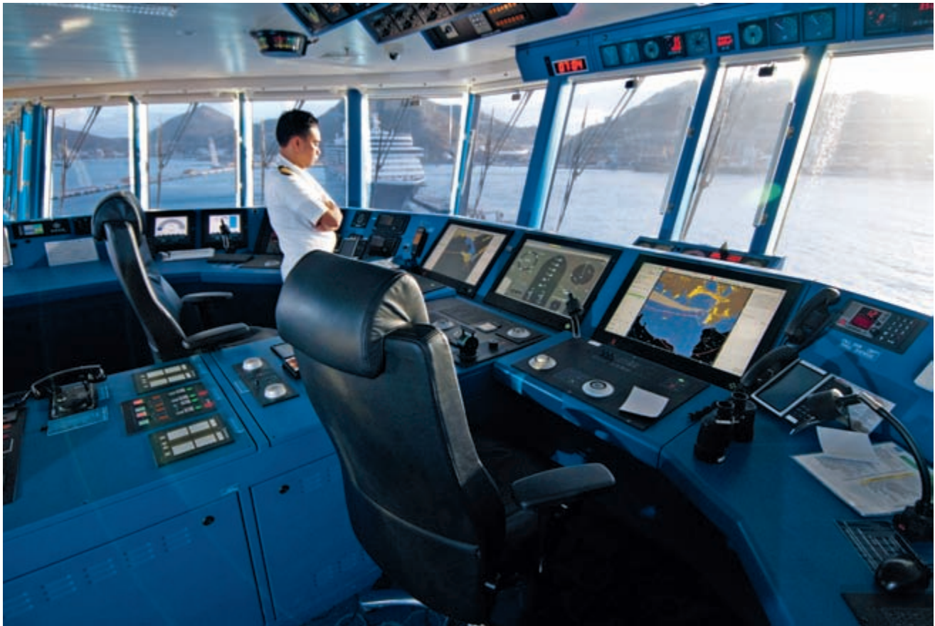
FIG. 504. INTEGRATED BRIDGE SYSTEM WITH ENC AND OTHER DISPLAYS.
