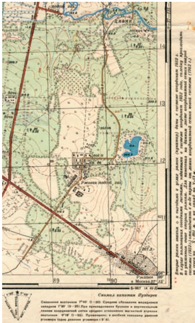
FIG. 575. DETAIL FROM THE FIRST EDITION OF THE 1:25,000 MAP (SHEET O-37-135-V-G, ALABUSHEVO). Drawn and printed in 1949 with the 1942-System. It demonstrates that at this scale the introduction of the 1942 coordinate system required more than simply changing the grid printed on maps. The marginal annotation shown indicates that the margins of this sheet had been shifted. It also states that to calculate a (Pulkovo) 1932 system coordinate value, the value of the 1942-System northing should be reduced by 801 meters and the easting reduced by 13 meters. Facsimile reprints of the adjacent sheets (still constructed on the Pulkovo 1932 system) nevertheless continued into the mid-1950s. The area shown includes the Moscow-Leningrad highway to the west of what is now Moscow's Sheremetyevo International Airport. Size of the entire original: 42.5 \times 35 cm; size of detail: ca. 22.4 \times 13.5 cm. Image courtesy of John L. Cruickshank.
