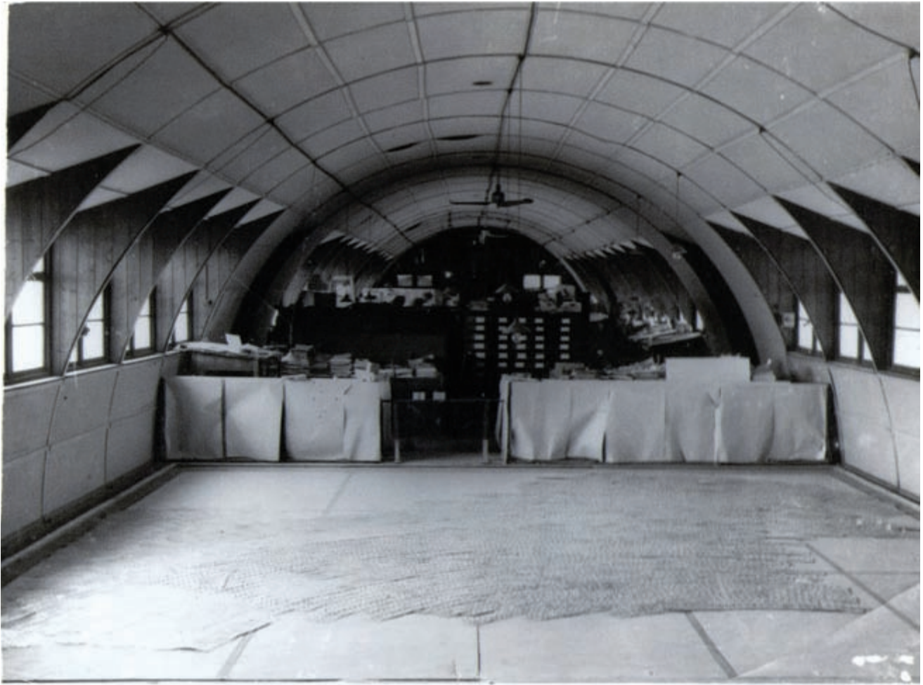
FIG. 547. SLOTTED TEMPLATES BEING USED IN 1948–49 FOR MAPPING JORDAN. A total of 9,989 templates were used in this survey, which covered Jordan and parts of Saudi
