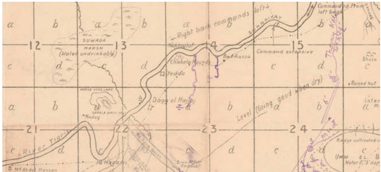
FIG. 595. DETAIL OF A TIGRIS CORPS MAP PRODUCED FROM AERIAL PHOTOGRAPHY. Sketch Map of the Country between Sheikh Sa'ad and the Shumran Bend , 1:126,720 (sheet T.C.4). Made for the attempted relief of the British forces besieged in Kut al Amarna, Iraq, this is believed to be
