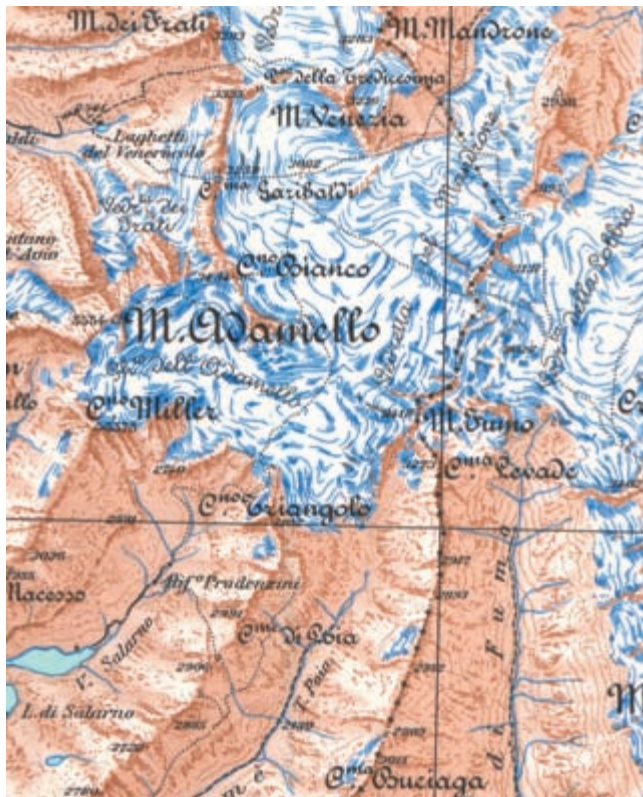
FIG. 562. DETAIL FROM M. ADAMELLO, 1950 (F. 20, ED. 4). This early edition, compiled in 1929 and updated in 1950, of the 1:100,000 series shows a mountain landscape characterized by glaciers, parallel ridge lines, and wide valleys. Size of the entire original: 46.2 × 52.8 cm; size of detail: 10.5 × 8.5 cm. Reproduced with permission of the Istituto Geografico Militare, Florence (authorization n. 6785 dated 04.06.2014).
