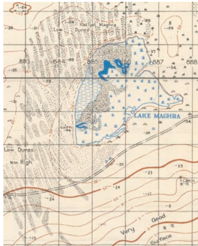
FIG. 582. DETAIL FROM EL MAGHRA , 1:50,000, 1942 (1st ED., SHEET 12). Part of the El Alamein position in Egypt, surveyed and drawn by the South African Survey Company in November 1941, it illustrates the difficulty in depicting desert landscapes using conventional line map methods. Size of the entire original: 57.0 × 42.5 cm; size of detail: 14.6 × 11.7 cm. Image courtesy of Peter Collier.
