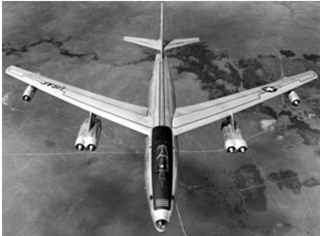
FIG. 534. BOEING RB-47E STRATOJET. The RB-47E was a photo reconnaissance version of the B-47E bomber and first flew in 1953. Used in the 1950s and early 1960s, they were lengthened by thirty-four inches to add an air-conditioned section for cameras. Their high speed and high altitude extended the range of aerial reconnaissance. Image courtesy of the National Museum of the U.S. Air Force, Dayton.
