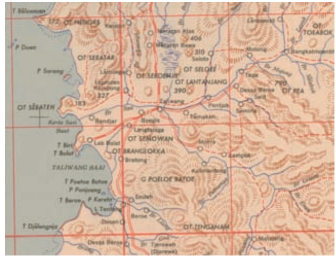
FIG. 598. DETAIL FROM MATARAM, LESSER SUNDA ISLANDS, 1:250,000, 1945. The map (Hind 1120, sheet 1, 2d ed.) was compiled by the U.S. Army Map Service from a variety of earlier Dutch sources. The Dutch had only carried out reconnaissance surveys, hence the use of hachures for relief portrayal.
