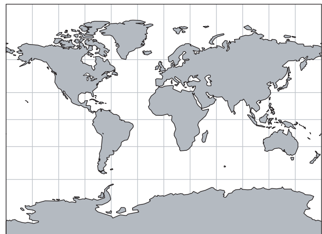
FIG. 603. MILLER CYLINDRICAL PROJECTION. Conceived as a modification of the Mercator projection, the Miller cylindrical projection sacrifices conformality (true angles) for substantially reduced areal distortion in polar regions.
